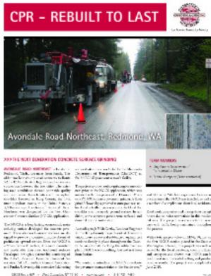
In this new case study, the King County Department of Transportation decided to use this new technique on Avondale Road Northeast in Redmond, Wash. The Next Generation Concrete Surface (NGCS) application was used since it is a long-lasting, economical, noise reducing surface for concrete pavement. The diamond saw-cut surface is designed to provide a consistent
