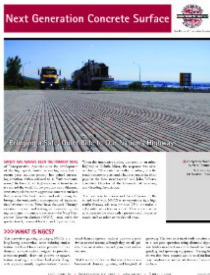
IGGA has recently released an FactSheet to address concerns over pavement noise. The new FactSheet explains the benefits of using the new Next Generation Concrete Surface (NGCS). NGCS is a grinding technique that results in a smooth and very quiet concrete surface, with improved friction properties at the same time. Concrete pavements also stay
